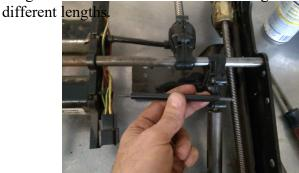
5. After removing the 4 screws from the casing With the bad gears, use a small screw driver to separate the two case halves.
